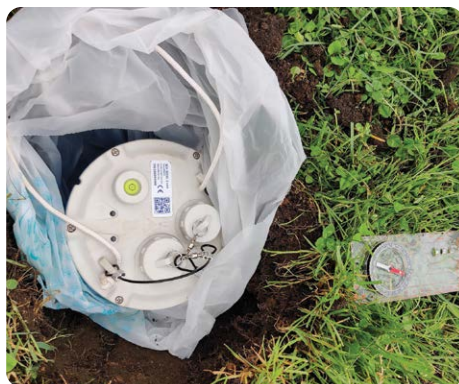
147 buried seismometers recorded data for a month.
