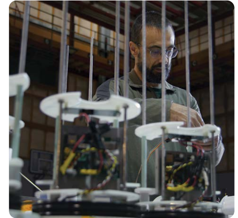
Neville Palmer prepares seafloor pressure sensors.
